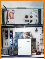
Test chamber for ozone test
