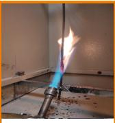
Propagation of vertical flame on complete single cable (acc. to EN 60332-1-2)
